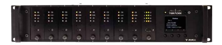
With room for up to 8 blades, T-Rax is the most powerful and affordable IP video solution for broadcasters and production companies. Combined with the Core Cloud Management Platform, T-Rax encoders and decoders can be managed remotely and routed to any number of destinations around the world, including decoders, online video platforms, and computers.
